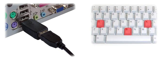
To record keystrokes, plug the device in-between the keyboard and USB port.
