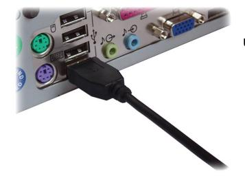
Disconnect the USB keyboard from the USB port at the computer or hub. This can be done even with the computer up and running.
